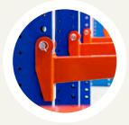
Cantilever Arms are connected to the upright columns with pivot pin system to prevent forklift damage when loading/unloading the level below; whilst maintaining height adjustability. They also come fitted with a removable end stop pin.
