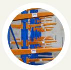
Cantilever Arms are connected to the upright columns with a pivot pin system to prevent forklift damage when loading/unloading the level below; whilst maintaining height adjustability. They also come fitted with a removable end stop pin.
