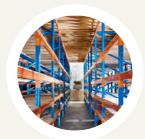
Rack Supported Raised Storage Areas use the racking structure to support the raised area, platforms can be created to allow for picking on several levels.
